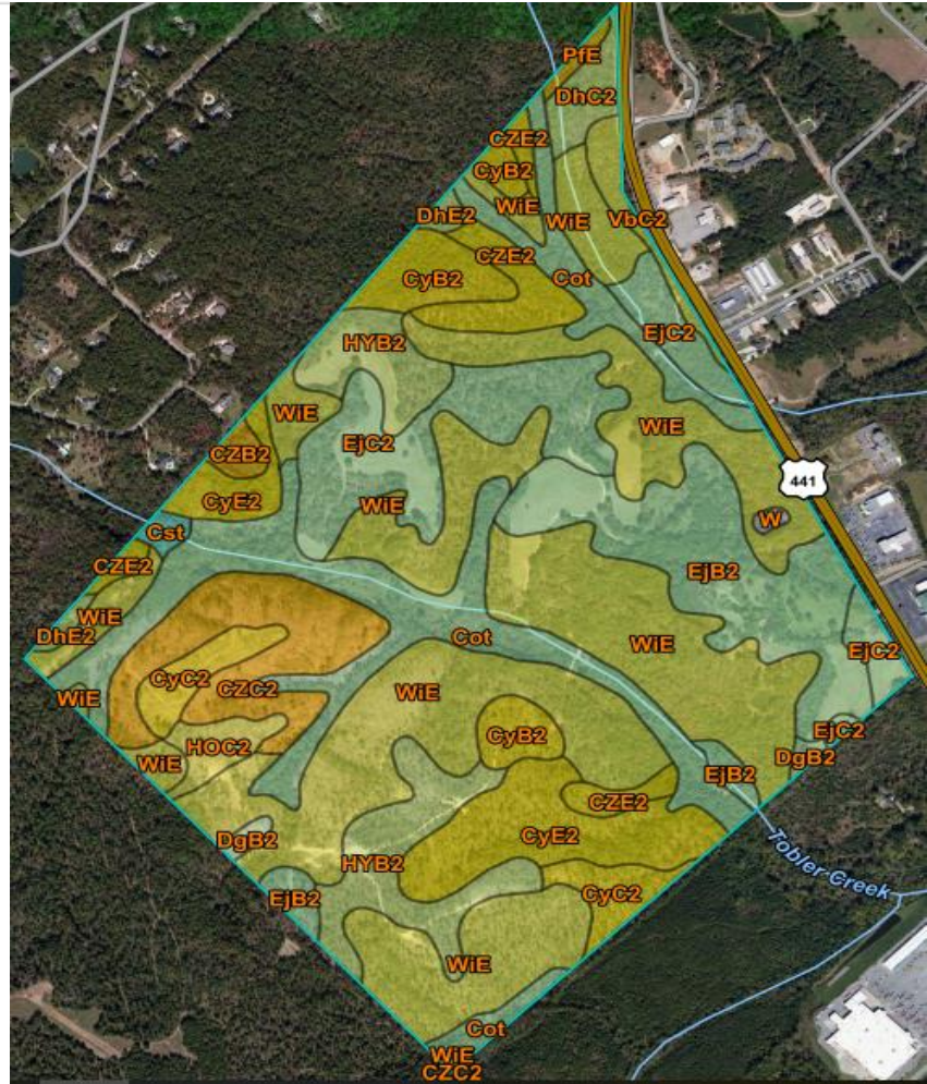
Fig. 13. Description Erosion factor K indicates the susceptibility of a soil to sheet and rill erosion by water. The estimates are based primarily on percentage of silt, sand, and organic matter and on soil structure and saturated hydraulic conductivity ( K_{sat} ). Values of K range from 0.02 to 0.69. Other factors being equal, the higher the value, the more susceptible the soil is to sheet and rill erosion by water.
