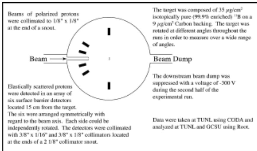
**FIGURE 1.** *Schematic layout for the experiment.*
