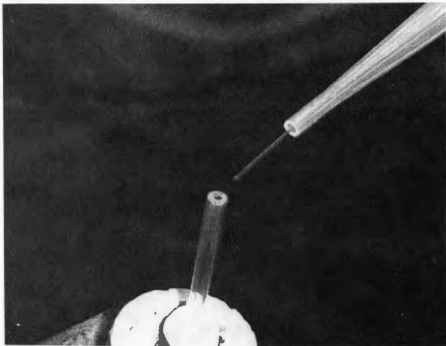
Figure 3. The angle created between the argon gas flowing through a GC column and the microphone. The angles are varied using an articulating mounting device and the resulting frequency is recorded.
