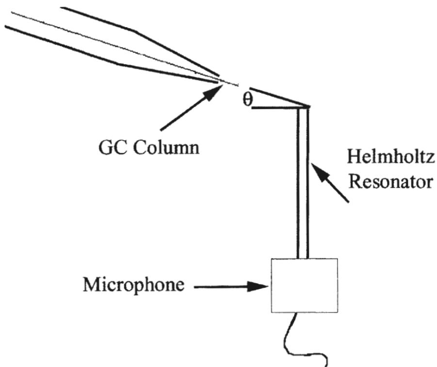
Figure 4. The pipette was supported by the articulating mounting device, which created an angle relative to the x-axis.
