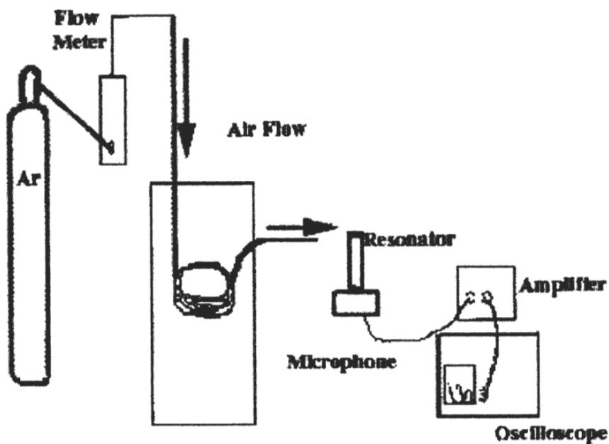
Figure 2. A constructed model of a Helmholtz resonator apparatus. Argon gas flows through a GC column to a sensitive microphone. The microphone is connected to an oscilloscope and an amplifier, which measures the frequencies.
