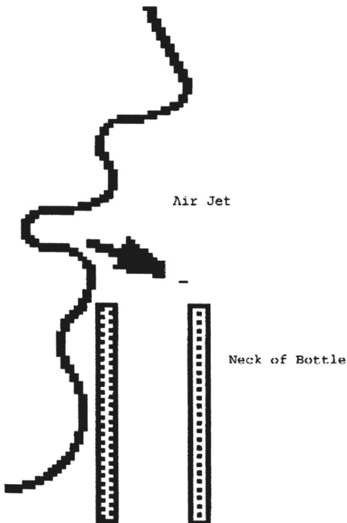
Figure 1. A simulation of a person blowing air around the neck of a bottle that creates a whistling noise. This is an example of a Helmholtz resonator.
